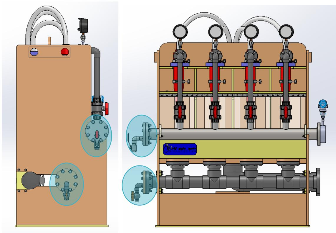
Figure 14 – Flush ports from top to bottom: Feed, Underflow
