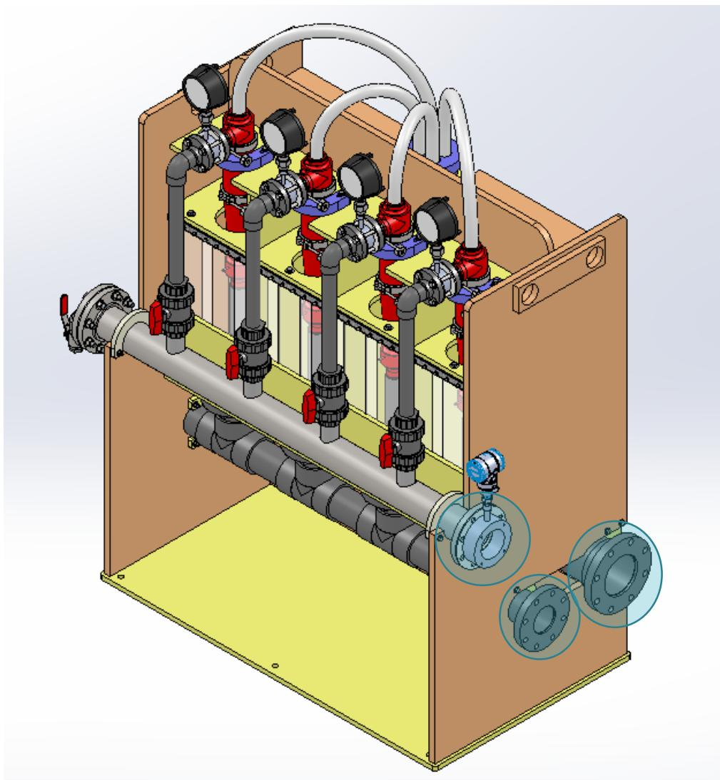
Figure 10 – Inlet and outlet flanges for process connections from left to right: Feed, Underflow, Overflow
