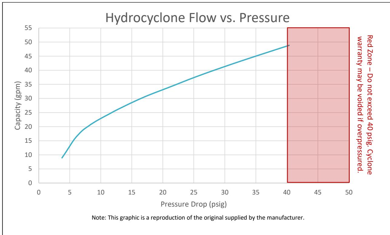
Figure 2 – Cyclone Performance Curve
