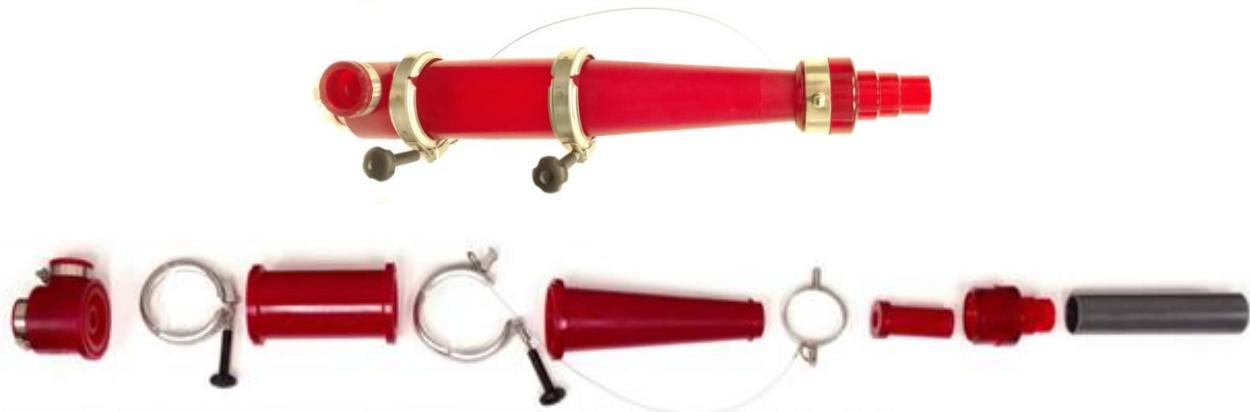
Figure 18 – Assembled (top) and disassembled (bottom) hydrocyclone assembly. In order from left to right: vortex finder with t-bolt clamps, v-clamp, body extension, v-clamp, main body, retainer ring, spigot (tip, nozzle, etc.), spigot retainer cap, spray guard.
