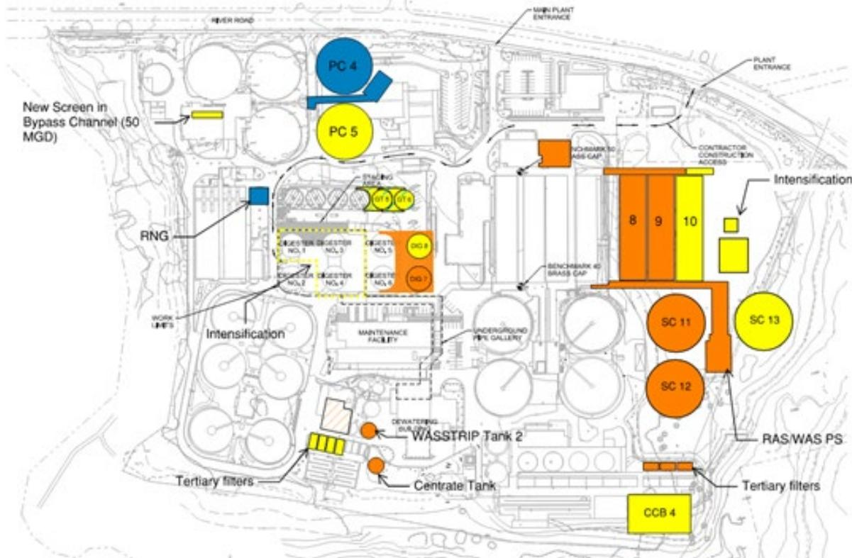
Figure 4.3 Rock Creek Site Layout (based on original Intel growth projections)
