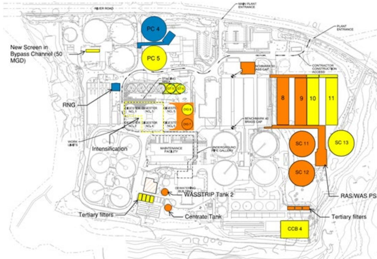
Figure 4.4 Potential Rock Creek Site Layout with Conventional Secondary Expansion Including Larger Aeration Basins and Secondary Clarifiers
