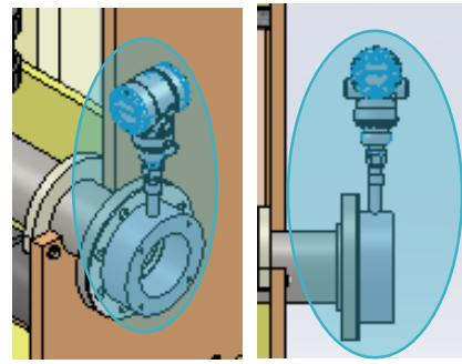
Figure 9 – Influent Pressure Transmitter with Isolator Ring
