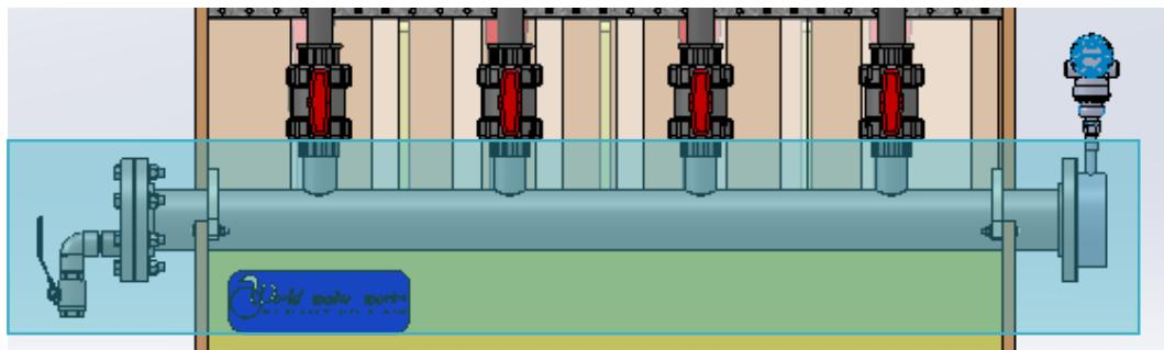
Figure 11 – Feed Manifold
