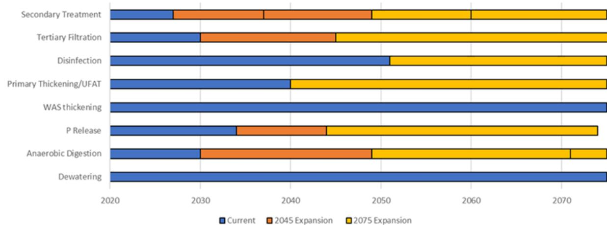
Figure 4.2 Rock Creek Capacity Limitations (based on original Intel growth projections)
