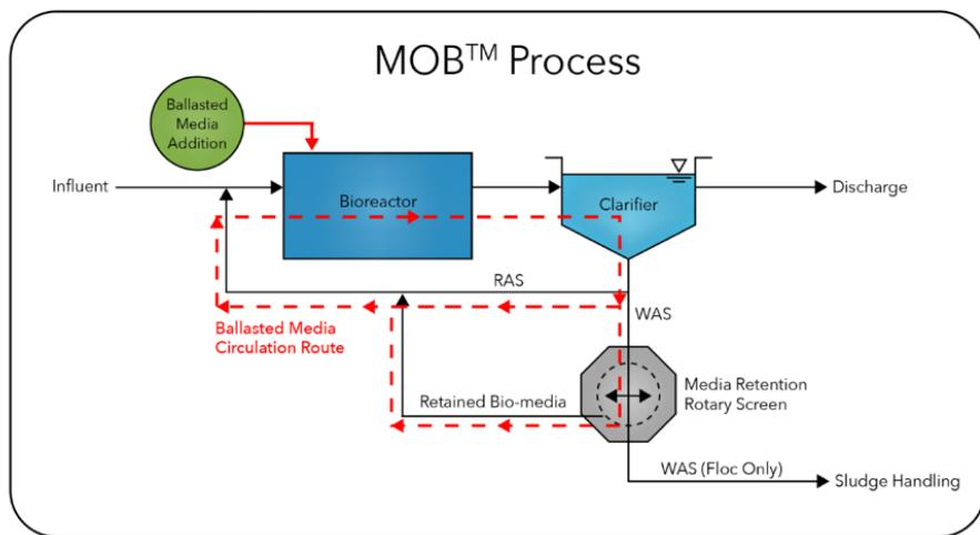
Figure 1. MOB™ Process Flow Diagram.
