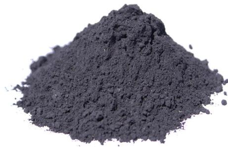
**Figure 2: Sample of magnetite material used with the BioMag system.**
