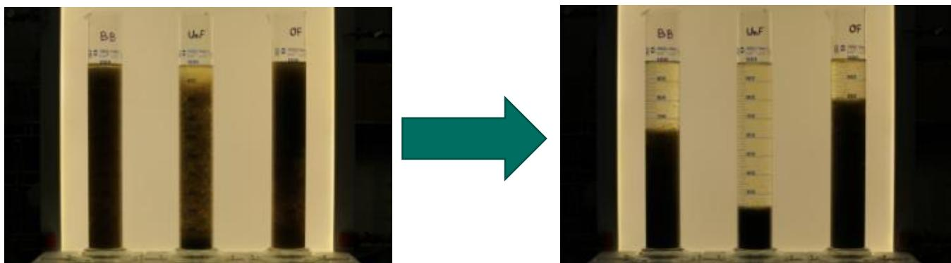
Figure 19 – Each picture has three cylinders with the Feed (F), Underflow (UF) and Overflow (OF) from left to right. The photo to the left is at time = 0 min and the photo to the right is at time = 5 min.
