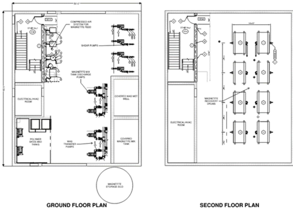
Figure 4.8 BioMag® Building Layout
