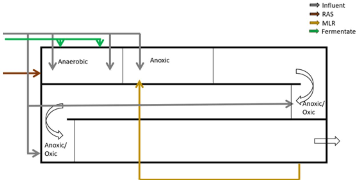
Figure 4.6 Preferred Configuration for the New Rock Creek Aeration Basins
