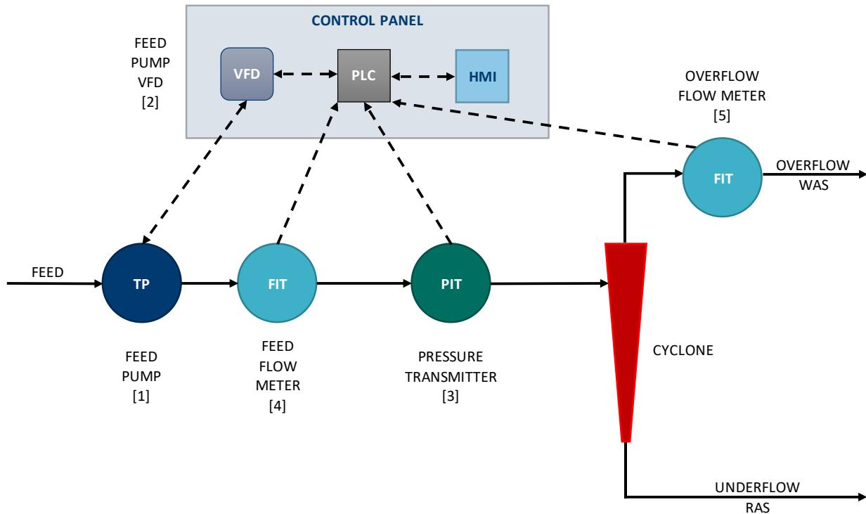
Figure 4 – Basic Process Flow Diagram with Instrumentation
