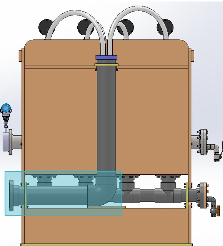
Figure 13 – Overflow Manifold
