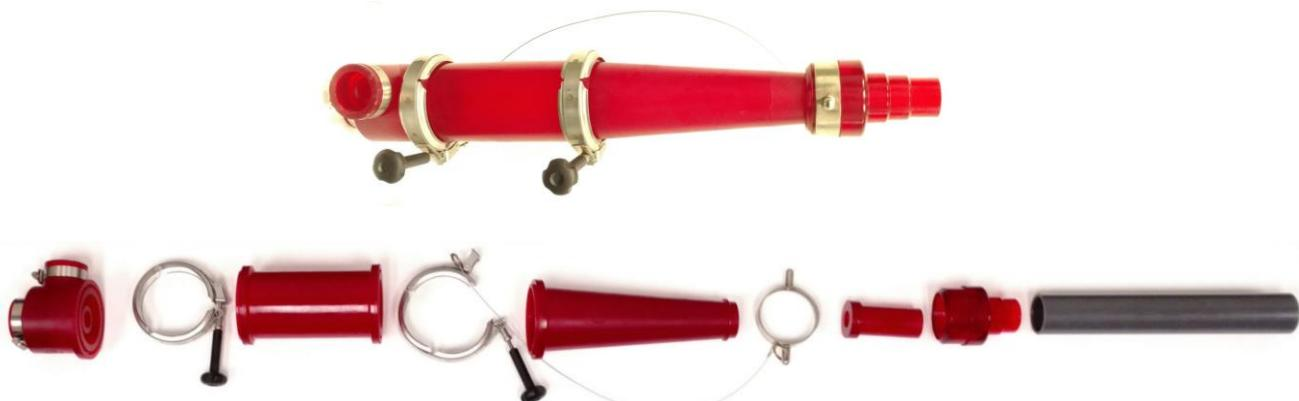
*Figure 5 – Assembled and disassembled hydrocyclone assembly. In order from left to right: vortex finder with two t-bolt clamps, v-clamp, body extension, v-clamp, main body, retainer ring, spigot (tip, nozzle, etc.), spigot retainer cap, spray guard.*
