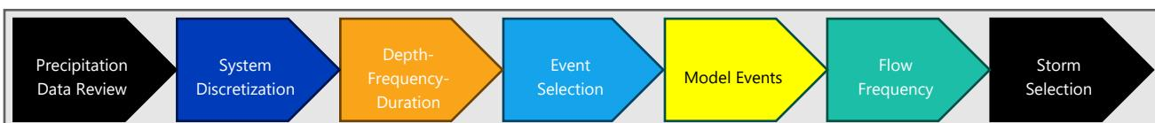
Figure 2.2 Methodology for Design Storm Development
